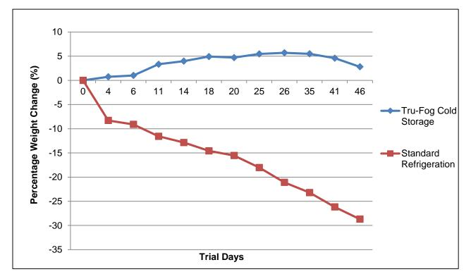
After 46 days: Samples in Pendred Tru-fog cold storage increased in average weight by 3% compared to Standard refrigerated cold storage where samples decreased in average weight by 29%.
